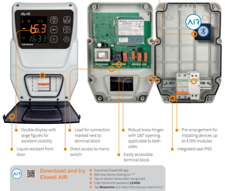
Line of electronic controllers for single-phase cold rooms, with direct control of compressors up to 2 HP, evaporator fan, defrost heater, cold room light and alarm.
