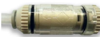
Put the core back in place and close the filter. Note the direction of air flow (towards the sensor). Open the regulator on the gas cylinder and let the gas flow for approximately one minute without the calibration adapter connected to the sensor, then close the regulator.
